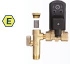
Great Lakes dryers utilize high quality diaphragm type solenoid valves as drains in addition to an isolation valve and strainer. Diaphragm valves isolate contaminants from the internal piston that would normally foul and restrict it's movement causing failure. Diaphragm valves also have much larger orifices and flow paths that in conjunction with the strainer virtually eliminates the possibility of clogging a condensate drain valve.
