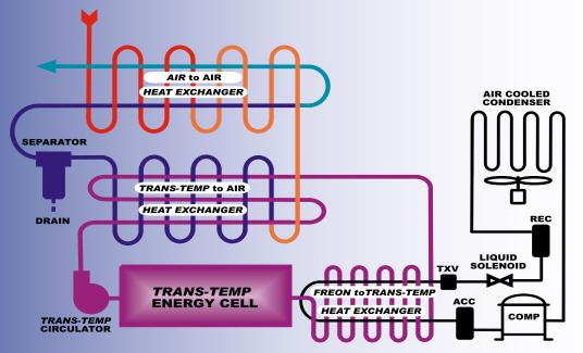
The **Trans-Temp Energy Cell**<sup>™</sup> integrates a proprietary blend of non-hazardous, completely biodegradable fluids that attains an ideal balance of thermal storage and thermal conductivity. The energy cell is encased in a heavy duty non ferrous vessel that is insulated to maintain energy efficiency.
